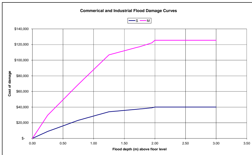
■ Figure 10-2: Commercial and industrial flood damage curves
